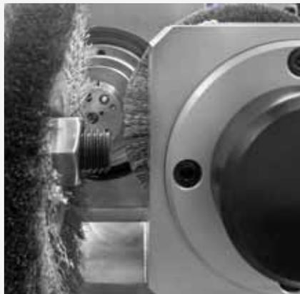
Simultaneous face and outside diameter brush deburring
