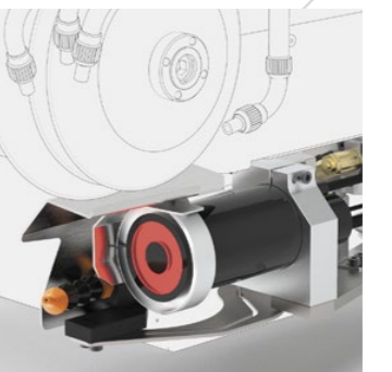
8. Vision system to locate miniature coolant holes
