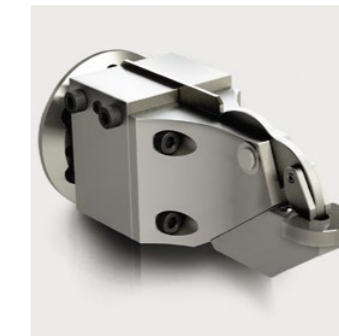
Claw clamping with platform for milling inserts
