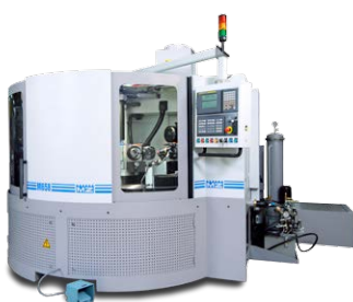
M658 2-station polishing machine for heads and inserts ■ Station 1: Polishing of head and inserts Station 2: Polishing of radius, chamfer, face
