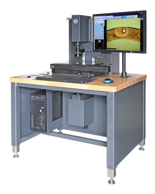
Marcel Aubert SA developed the George concept to control simultaneously both sides of a workpiece. The system works with one referential for both view (upper and downer). The workpiece can thus be checked, without any special holder, by defining the measurement references on the opposite side to the one to be controlled.
