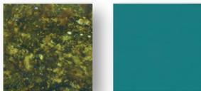
Metalworking fluids lose valuable cooling and lubrication properties when contaminated with oil and fines. Part quality and tool life are drastically compromised.
